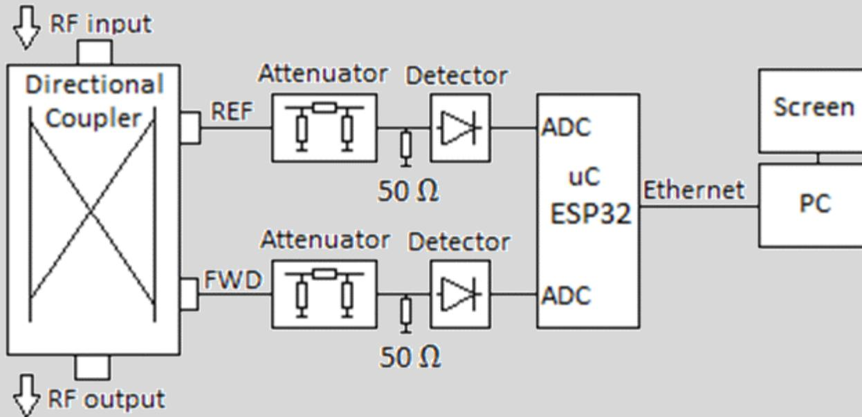
The RF signals decoupled from the directional coupler are passed via attenuators to detectors. These convert the RF signals for forward FWD and reflected REF into DC voltages, which are then digitised by means of AD converters (ADCs).
