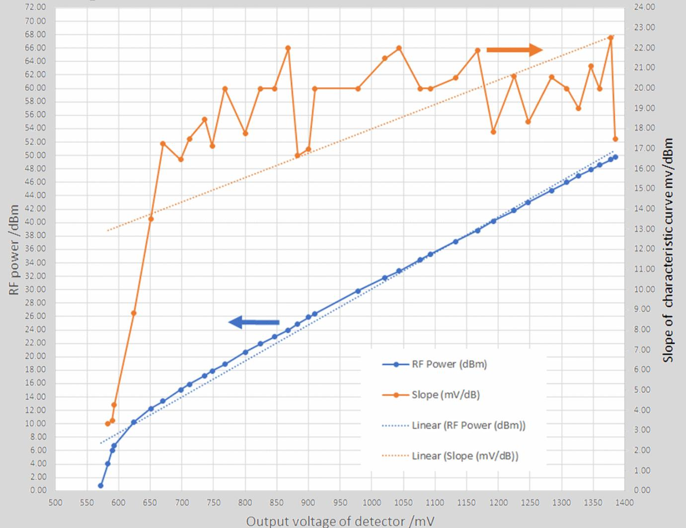
Example of the characteristic curve of the setup measured at 145 MHz. The maximum power of 50 dBm (100 W) was limited by the output power of the transmitter used.
