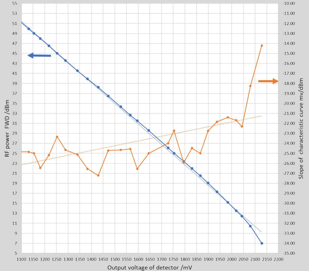
Example of the characteristic curve of the setup measured at 145 MHz. The maximum power of 50 dBm (100 W) was limited by the output power of the transmitter used.
