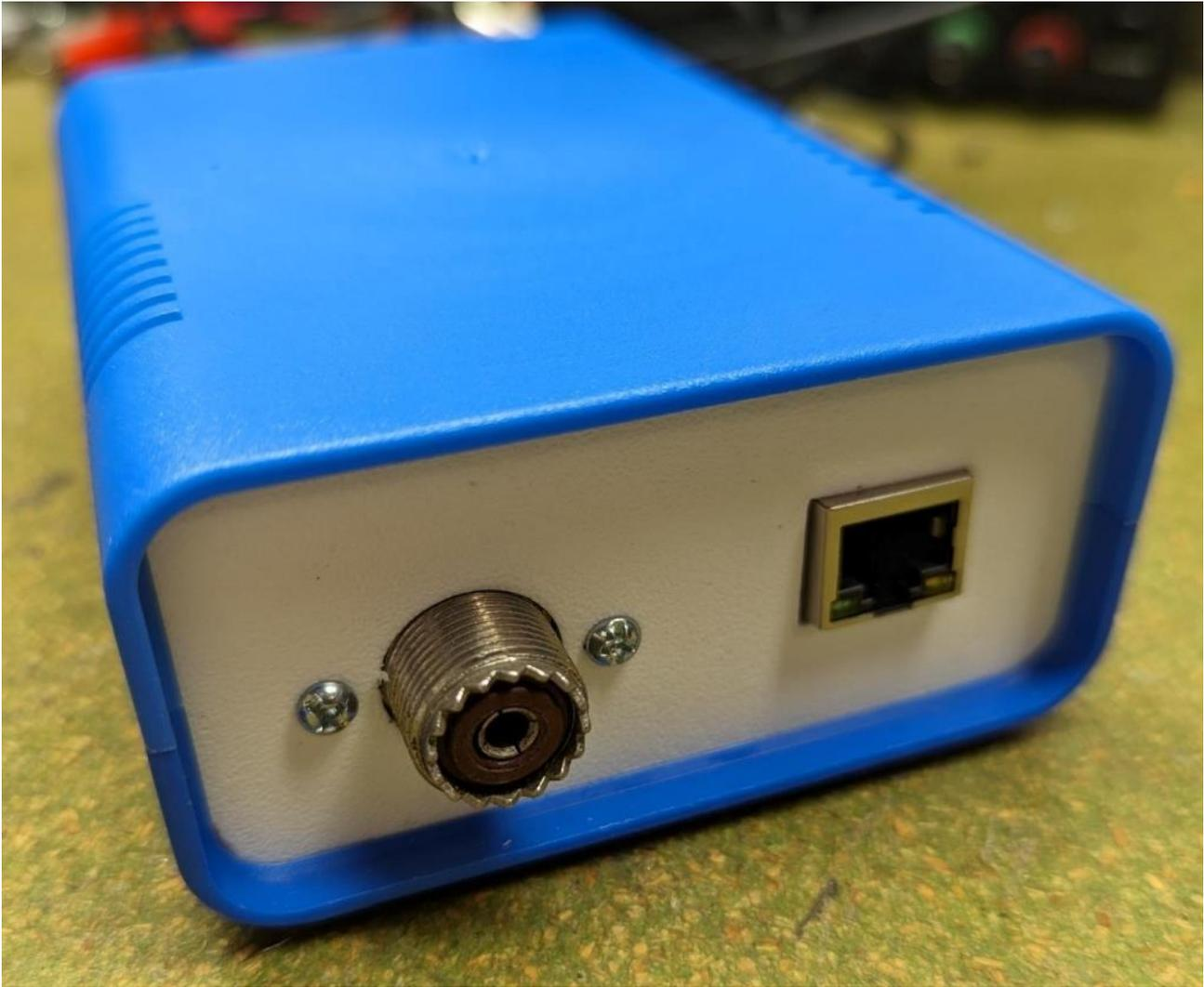
Figure 29: Front panel and rear panel were produced using 3D printing
