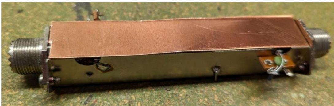
Figure 26: Disassembled directional coupler with additional shielding
