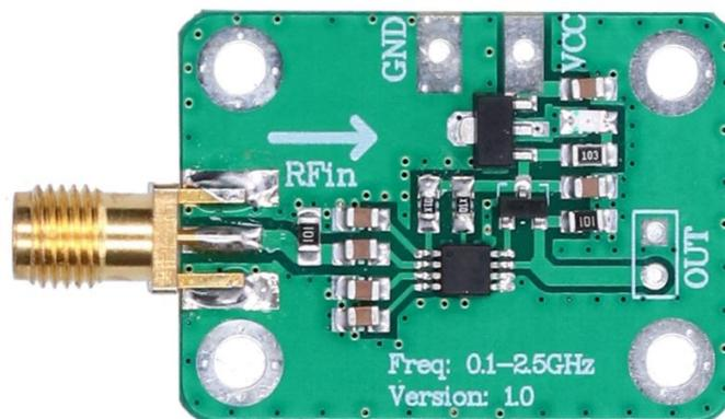
Figure 20: Detector board with AD8313
