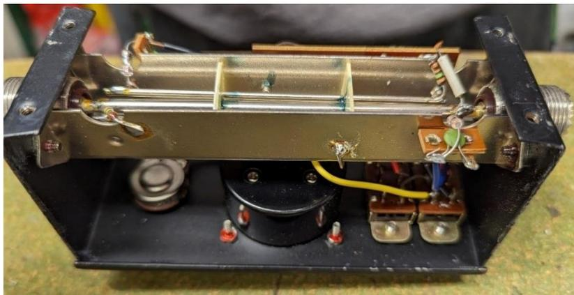
Figure 25: A directional coupler with integrated detector diodes is found in the VSWR meter
