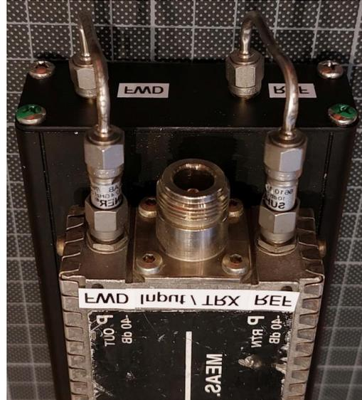
Figure 16: Back of the Remote VSWR & Power Meter
