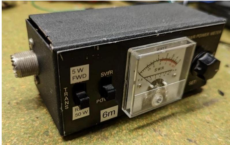
Fig. 24: Old VSWR / power meter for short wave
